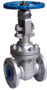
FIG. 272-CS-150 Class 150, Flanged ends, bolted bonnet, WCB body & bonnet, 13Cr/HF trim.
