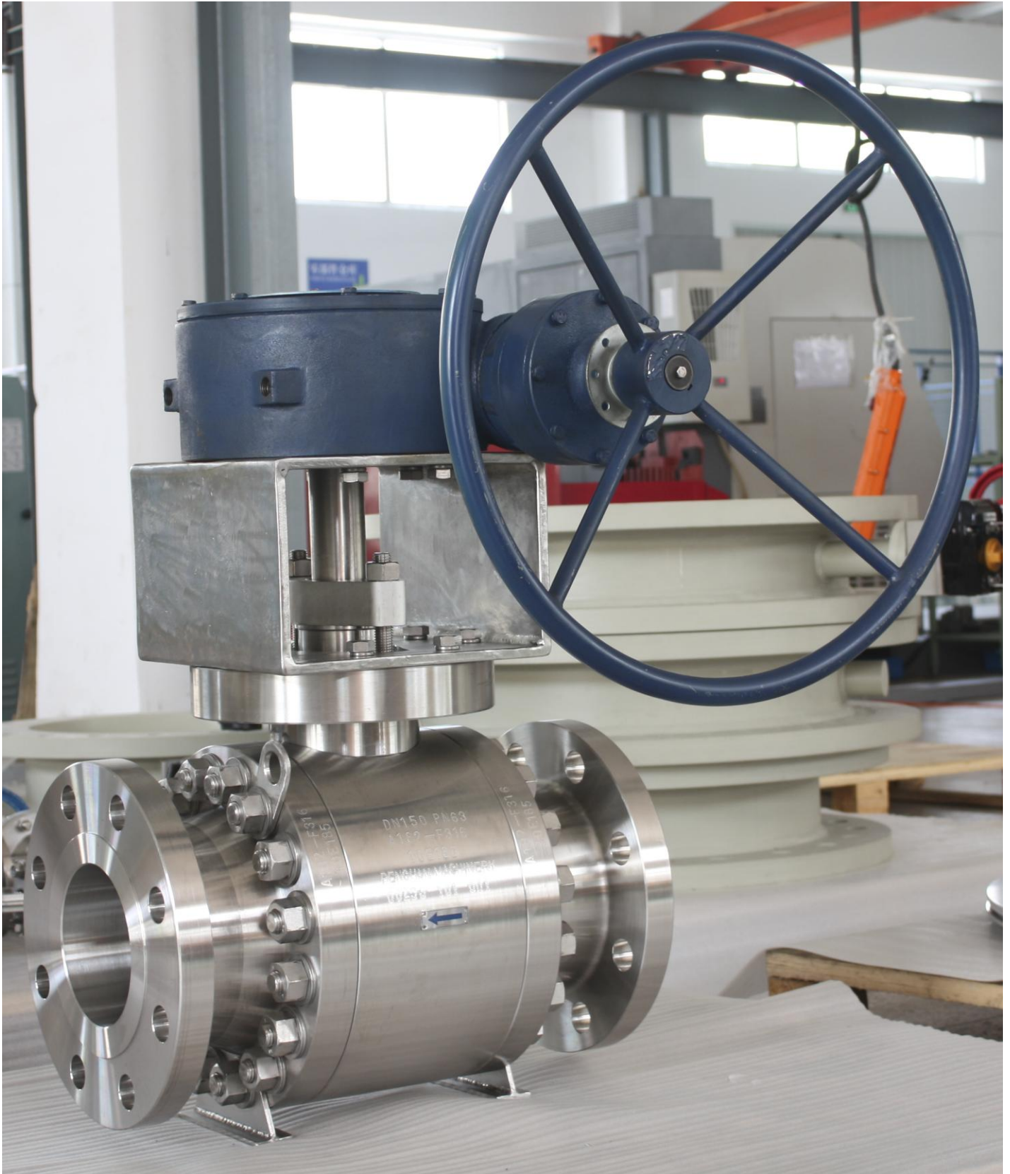
c) High Temperature Metal Seated Trunnion Mounted Ball Valve
