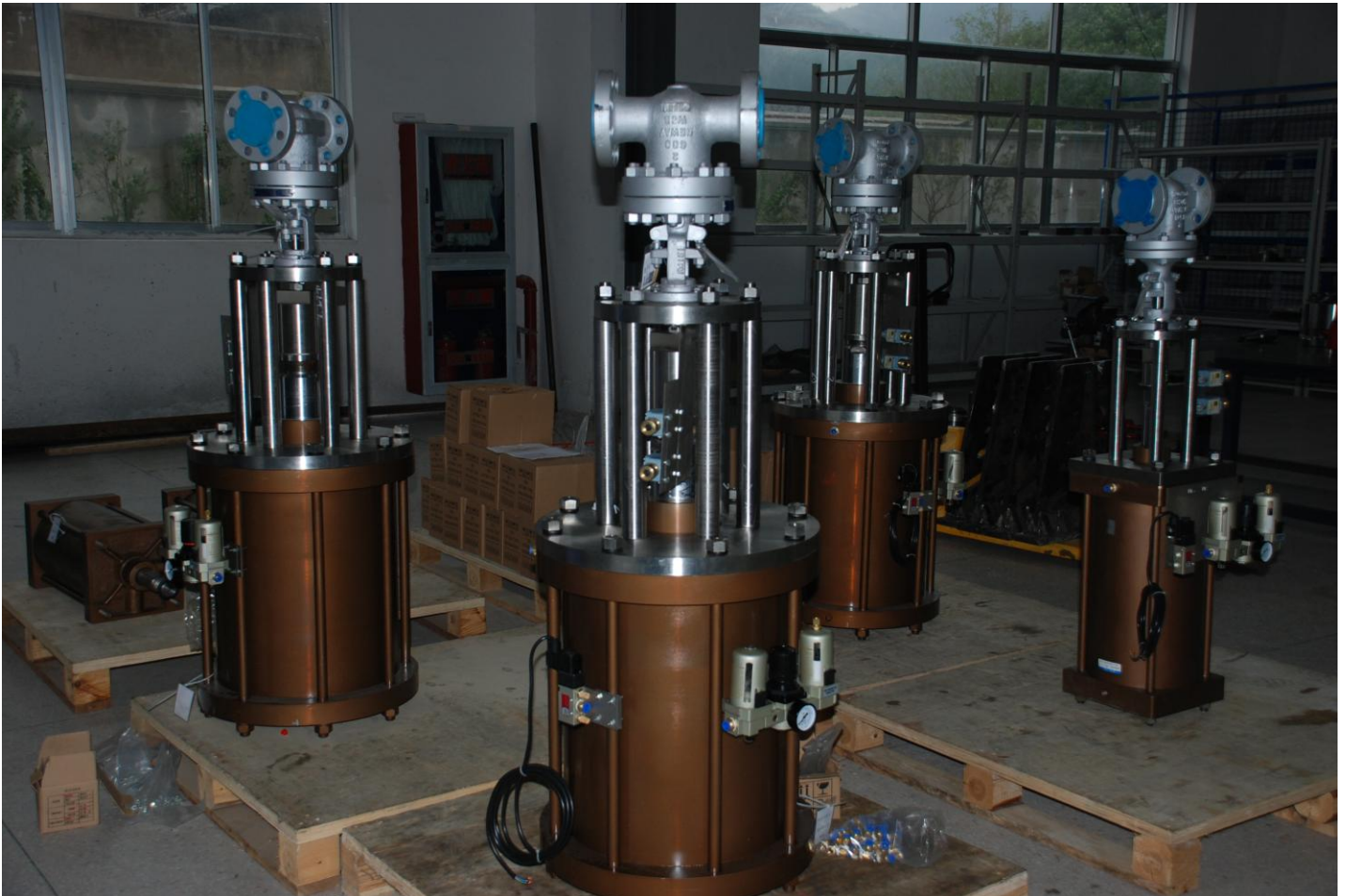
f) Pneumatic Gate Valve
