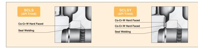
For KITZ cast steel valves made of ASTM A216 WCB, the standard shell material, disc seats and body seat rings shall be provided as follows. (Refer to Page 3 for Product Coding)
