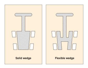
Heavily designed KITZ wedge gates are forged or cast solid, single piece of steel without any welding work. Specially heat-treated wedges are firmly coupled with integral T-head of the valve stems, which are also ruggedly designed and specially heat-treated for the highest possible durability of stem to wedge connection. API 600 Paragraph 5.8.7 particularly emphasizes the importance of the mechanical strength of this connection.
