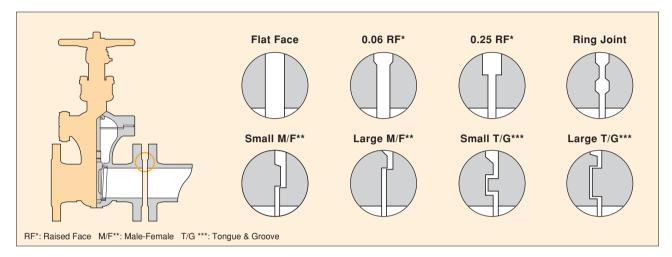
Gasket contact surface finish of end flanges as well as body-bonnet flange very much depends on the materials selected for flange gaskets.
